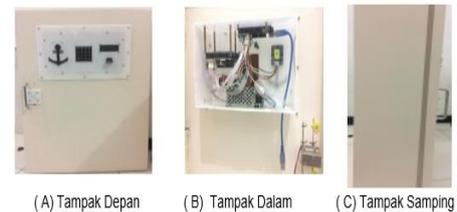
Design testing is done after the tool is finished. Testing is performed to see if the tool is working properly or not. Tests were also conducted to determine the durability of the device. The tool has been operating for more than 500 hours non-stop in standby mode to test which parts of the hardware are weak.
