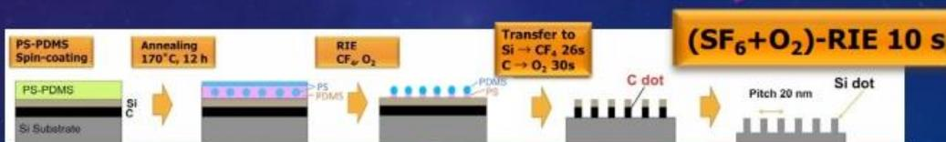
PS-PDMS Spin-coating → Annealing 170°C, 12 h → RIE CF<sub>4</sub>/O<sub>2</sub> → Transfer to Si → CF<sub>4</sub> 26s, C → O<sub>2</sub> 30s → (SF<sub>6</sub>+O<sub>2</sub>)-RIE 10 s
