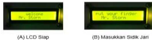
.When the user puts his finger on the fingerprint sensor there are two possibilities that the fingerprint is detected correctly (according to registration) or wrong. Hereis the result of fingerprint sensor testing.
