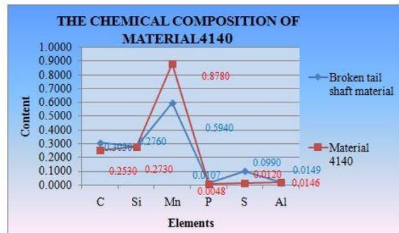
Fig. 9 Graph of chemical composition of material 4140
