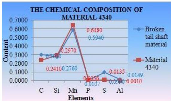
Fig. 8 Graph of chemical composition of material 4340
