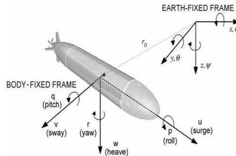
**Fig. 1.** Six degree of freedom of AUV motion
