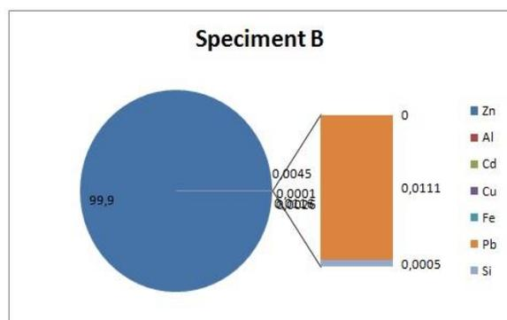
**Fig. 8.** Composition of Speciment B
