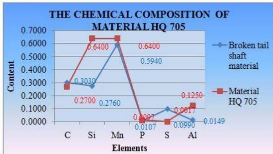
Fig. 7 Graph of chemical composition of HQ 705 material
