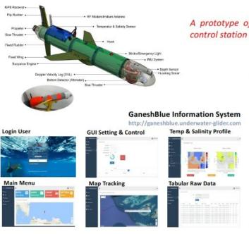
A prototype of underwater glider operated through ground control station using radio and/or satellite communication
