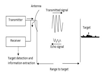
Fig 2.1 Radar Basic Principle (Skolnik,1962)
