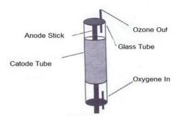
Figure 2.2. Reactor tube Model.
