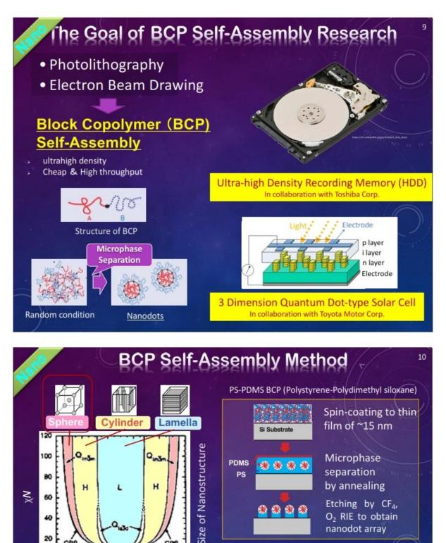
O<sub>2</sub> RIE to obtain 40 nanodot array 20 CPS The process to form PS-PDMS nanodot array DIS Ó 0.8 0.2 0.4 0.6 The ratio of PDMS fPDMS χ: Flory-Huggins Parameter, N: the total number of segments 1 cm<sup>2</sup> Si wafer DVD-sized Si wafer The theory of BCP Self-Assembly It is very easy to form monosize and monolayer nanodot array on high area
