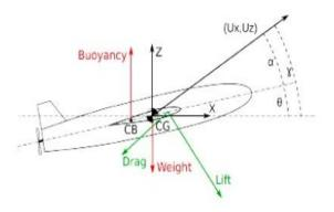
Fig. 1. Schematic representation of the principle of operation of an underwater glider.  $\theta$ ,  $\alpha$ , and  $\gamma$  are the pitch, angle of attack, and glide path angles, respectively (forces and moments exaggerated for clearer presentation).
