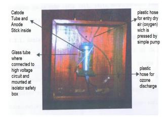
Figure 3.1. Reactor model
